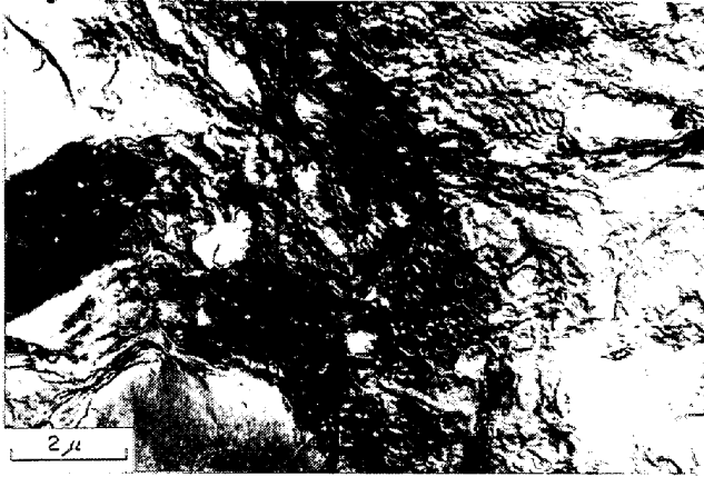
Photo. 7. Combined plastic-intergranular fracture in a specimen quenched and tempered at 200°C, near the original area of main crack nucleation.
