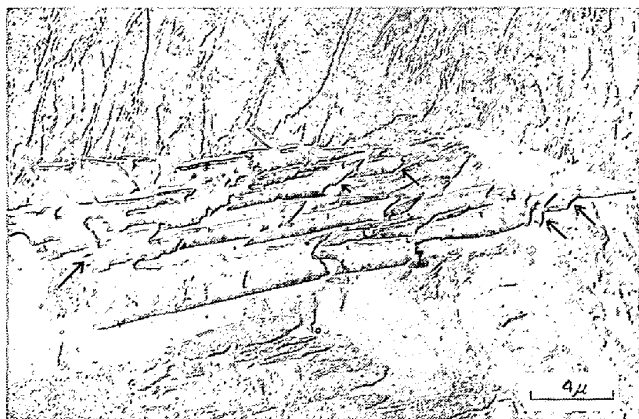
Photo. 10. The interface between the bainite formed at 450°C and the untransformed austenite in the Cu-Ni-Cr-Mo steel containing 0.22% carbon.
