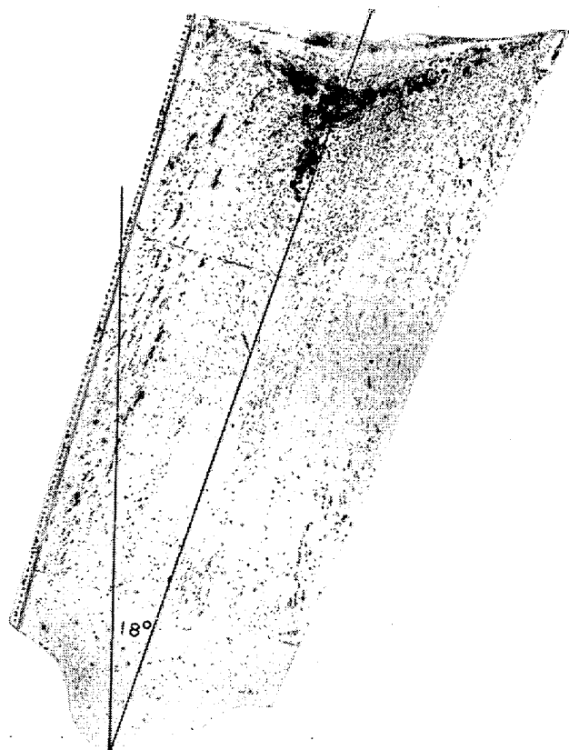
Photo. 7. Sulfur print of 1.3 t steel casting solidified at inclined state with angle of 18° to the axis.
