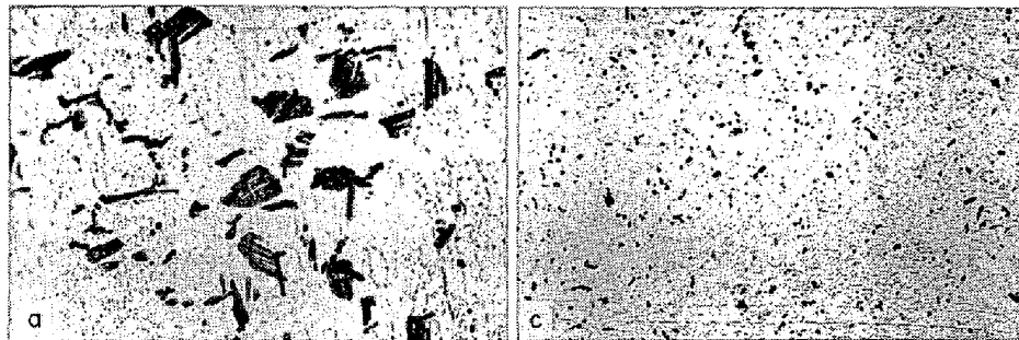
Photo. 3. Electron microstructures of 22 Cr-12 Ni series tested at 650°C.
