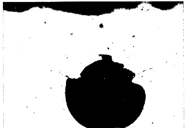
Photo. 3. Crack initiated from the blowhole. \times 100 (3/5)
