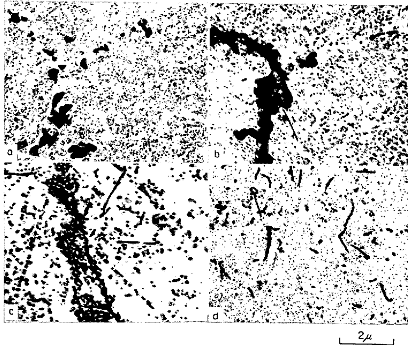
Photo. 3. Electronmicrostructures of creep-ruptured specimens of the steel C10B9, (extraction replica).
