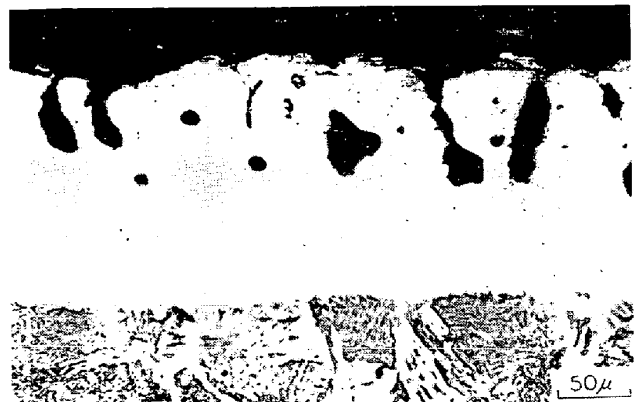
Photo. 3. Porous phosphorized layer treated in molten salt of \text{NaPO}_3 60%, \text{NaCN} 10%, \text{Na}_2\text{CO}_3 26%, \text{NaCl} 4% at 950^\circ\text{C} for 6 hr.
