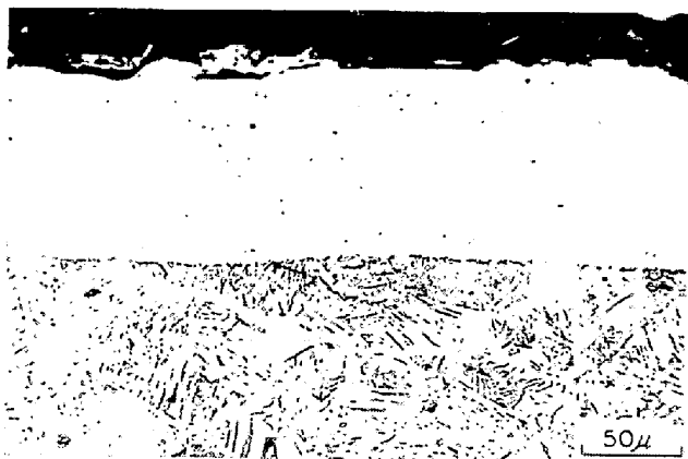
Photo. 4. Uniform phosphorized layer treated in molten salt of NaPO 3 40%, NaCN 5%, Na 2 CO 3 48%, NaCl 7%, at 950°C for 7 hr.
