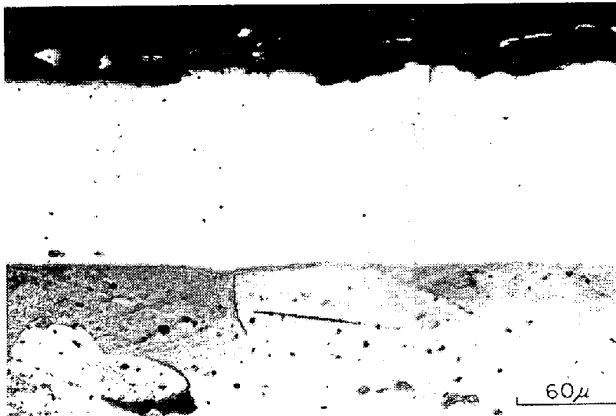
Photo. 1. Uniform phosphorized layer treated in ferro-phosphorous grains with few % of charcoal at 1000°C for 8 hr.
