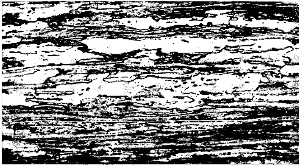
Photo. 1. Microstructure of the longitudinal section of the 80% cold-rolled Al-killed steel sheet after 1st-stage annealing at 560°C for 40 min. \times 600(1)
