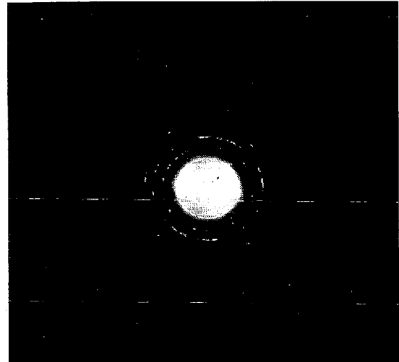
Photo. 1. Electron diffraction pattern of the oxide on the surface of liquid Fe-V containing 5.5%. (Identified as VO)
