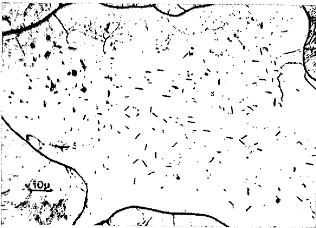
Photo. 2. Micrograph of a specimen annealed at 1200°C. (volume diffusion range) \times 1000(1/2)
