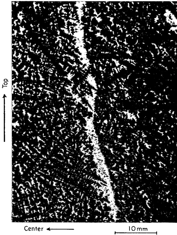
Photo. 9. An inverted V segregate showing fine internal structure in the 3 t test ingot. ( 198 Au)
