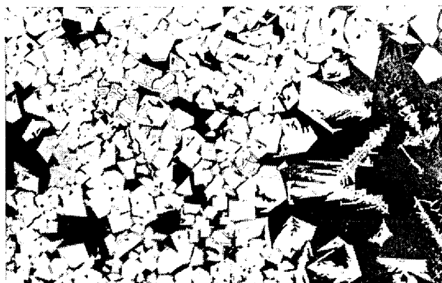
写真 3 Microstructure of sinter which is well assimilated. \text{CaO}/\text{SiO}_2 1.5, \text{SiO}_2 5.5% \text{Al}_2\text{O}_3 1.5%, \text{MgO} 1%
