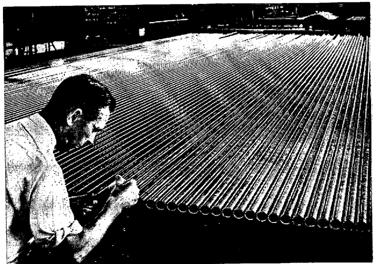
Photo. 9. Inspection of stainless-steel tubing.
