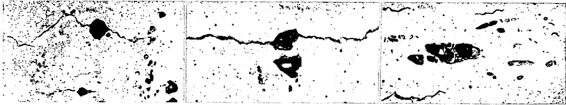
(a) Microcracks initiated from \text{Al}_2\text{O}_3 -type inclusions. 1.9 \times 10^6 cycles (b) Microcracks initiated from MnS-type inclusion fractured brittle. 1.16 \times 10^4 cycles (c) No microcracks initiated from MnO-type inclusions deformed ductile, where the rolling direction is transverse to the long axis of the specimens. 10^5 cycles
