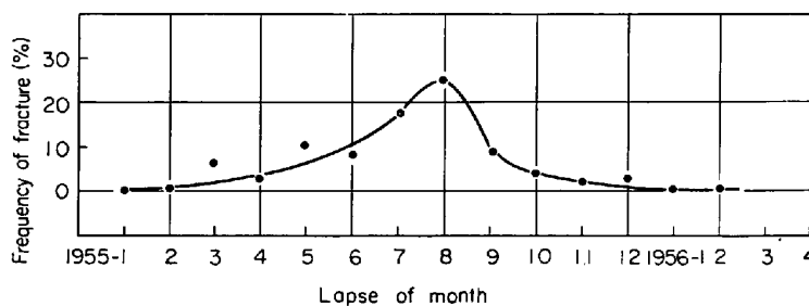
Fig. 8. Relation between frequency of fractures and melting period of the rolls.
