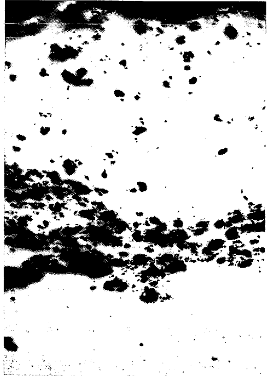
Photo. 6. The growth of the oxide inclusion in Fe-Ti alloy. \times 70 (2/3)
