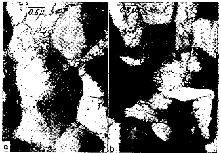
a: 650°C, 10.5 kg/mm 2 100 hr b: 650°C, 10.5 kg/mm 2 340 hr (ruptured)
