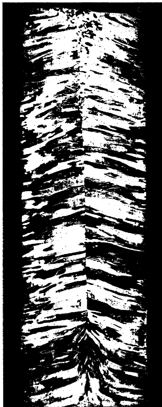
Photo. 1. Macrostructure of 180mm×850mm ingot. (×1/4)
