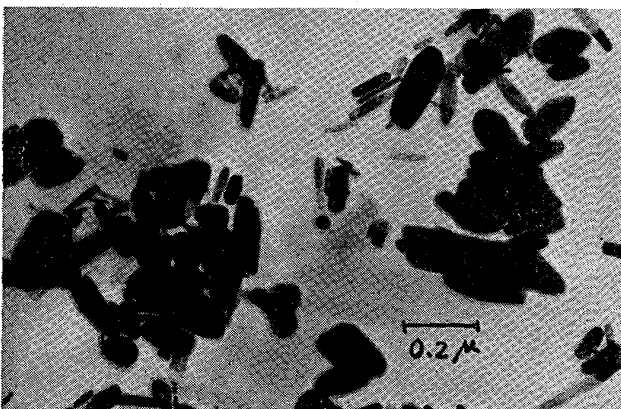
写真23 \text{Mo}_2\text{C} , 電解抽出残渣. ( \text{Mo}=2.6\% ) ×50000 (2/3)
