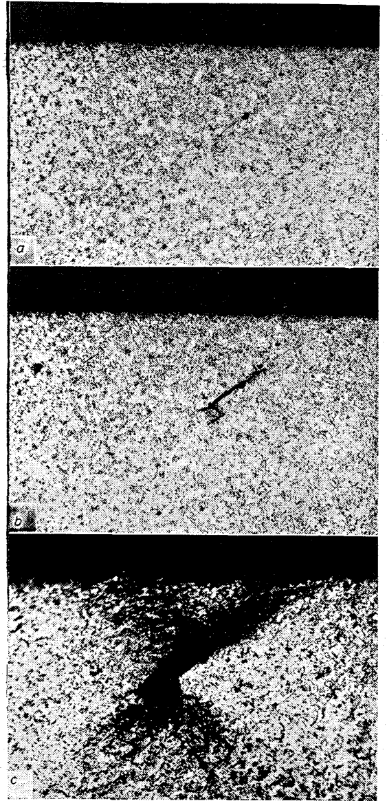
Photo. 3. The appearance and growth of crack from a non-metallic inclusion (silicate) by flattening test. (microscopic observation of cross section of tube)
