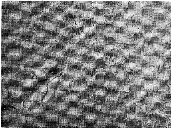
Photo. 5. Discharged surface of artificial defaced specimens. \times 5000(4/7)
