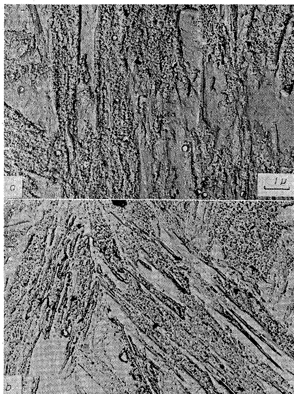
Photo. 1. Election microstructure of step quenched steel at 400^{\circ}\text{C} for 10min (a) and 1000 min (b).
