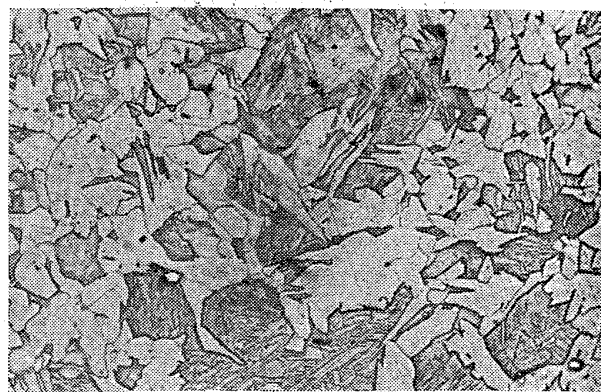
Photo. 1. Microstructure of \text{N}_2 steel which cooled continuously and then quenched rapidly from 653^\circ\text{C} , 10 sec.
