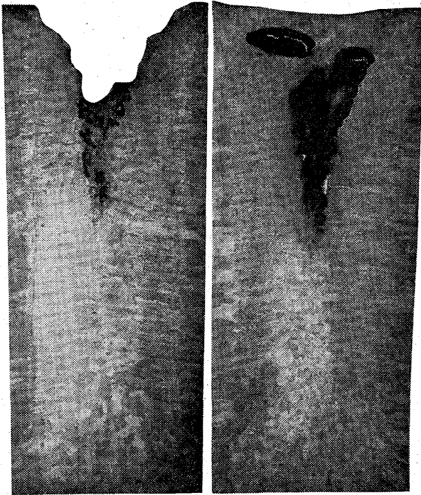
(a) Solidified under ordinary pressure (b) Solidified under pressure of 10\text{kg/cm}^2
