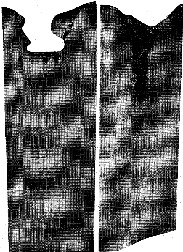
(a) Solidified under ordinary pressure (b) Solidified under pressure of 20kg/cm 2
