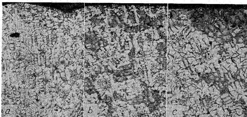
a) Melt 4 b) Melt 5 c) Melt 6 Photo. 3. Micro structure from Melt 4, 5, 6 after firing the glass. Etched in 4 per cent picral.
