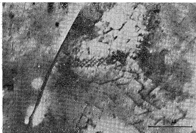
Photo. 1. Electronmicrograph of a low carbon mild steel which was deformed in tension (stress; 3.32 kg/mm 2 , strain; 0.02%).
