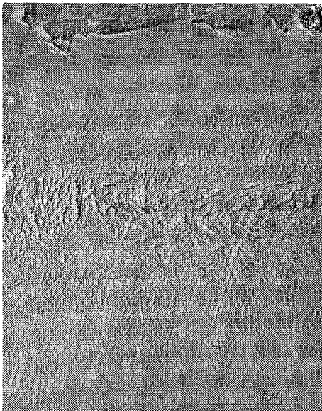
Photo. 3. Electron microscopic photograph in discharge crater (×4500) specimens-W.Q. (0.68%C). (1/2)
