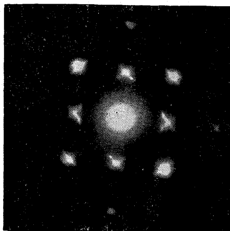
Photo. 12. Electron diffraction pattern of plate-like sulfide inclusions.
