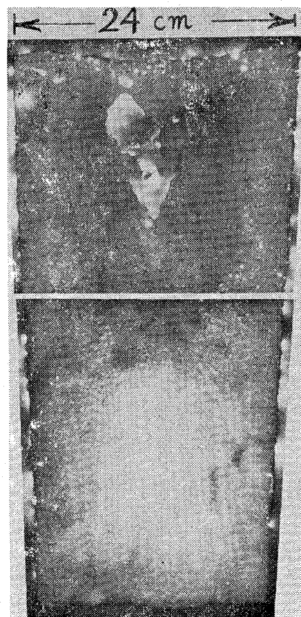
Photo. 3. Autoradiograph of longitudinal cross-section of 250 kg killed steel ingot; ^{140}\text{La} was added to ladle.
