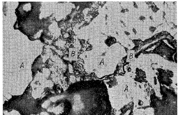
Photo. 1. Microscopic structure of a briquette. A=Iron sand, B=Iron oxide binder. ×600(1/2)
