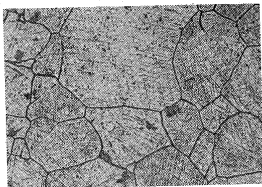
Photo. 2. Microstructure of 2 Mo-0.41 N aged at 900°C for 1 h after 1200°C solution-treatment. Etching solution: 1 HCl+1 alcohol. \times 100 (9/10)
