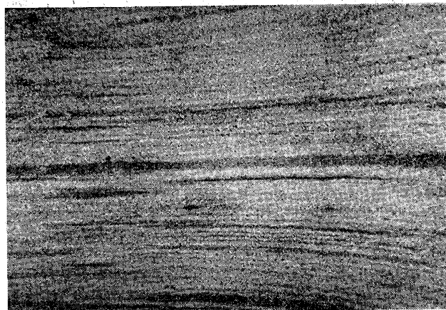
Photo. 1. Example of fibre structure as seen on the longitudinal section of a SKF 3/8 in. ball. ×50 (1/1)
