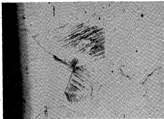
KXV 2 (Type 310) 1100°C×1h W.Q. \sigma_w = 14 \text{ kg/mm}^2 , N = 4.7 \times 10^6 10% oxalic acid, electrolytic etch, ×200
