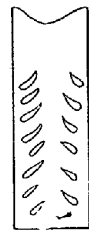
Fig. 11. Illustrating blow holes in a specimen cast in sand mould from a melt bubbled with water vapour. \times 1/2(2/5)
