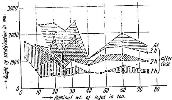
Fig. 6. Relation between nominal ingot size and solidification height in early hours after cast.
