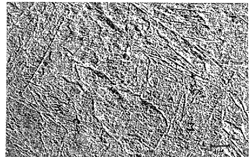
Tempered at 230°C for 20 mn. after quenching. C : Cementite, C' : flaky cementite, M' : Tempered martensite
