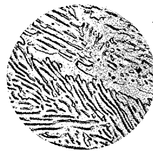
×5,000, (2/3) picral etch Fig. 10. Microstructure of billets with low-hydrogen content. (bearing steel)
