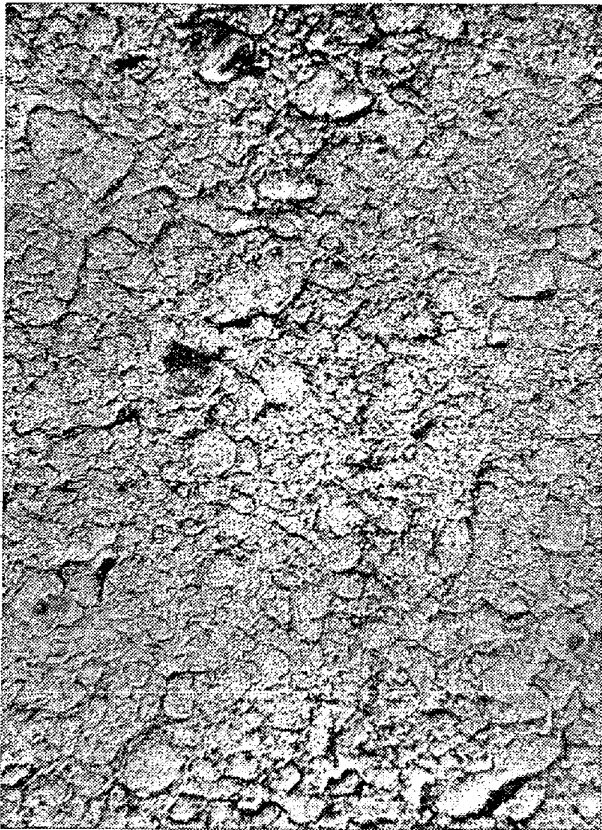
Photo. 2. Tempered at 360°C acetylcellulose-aluminum filmy replica shadowed with Cr.
