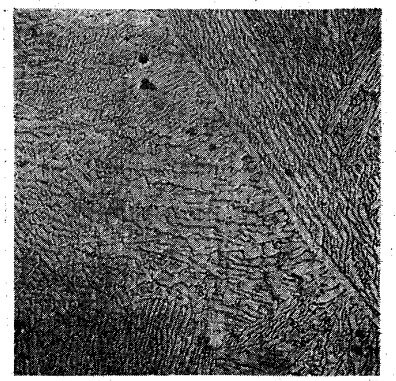
F 18.5 \begin{pmatrix} Ni & 7.5\% \\ Cr & 18.5\% \\ Fe & 74\% \end{pmatrix} 爐中冷却 ×100 No. 30
