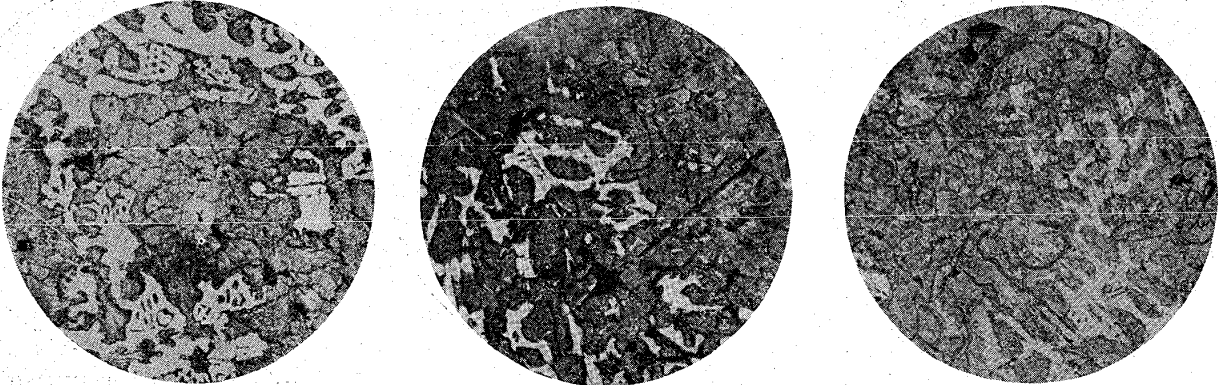
Fig. 18. (1-6) Effect of the Silicon content on the graphitization of white pig iron melted at 1,450 °C
