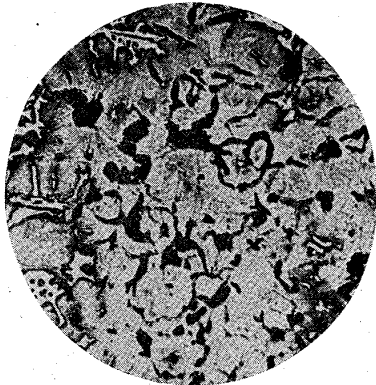
Fig. 20. (1-5) Effect of Mangan content on the graphitization of low Silicon white pig iron melted at 1,400 °C (1) Si:0.475 Mn:0.441 (2) Si:0.479 Mn:0.543 (3) Si:0.488 Mn:0.735
