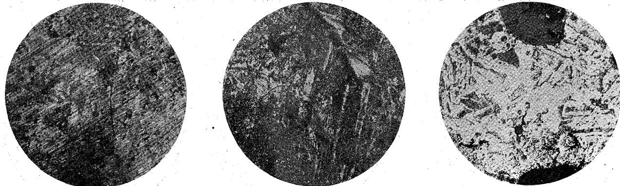
Fig. 14. (1—4) Microstructures of iron for different length of time of reduction at 1,400 °C with eutectic slag.
