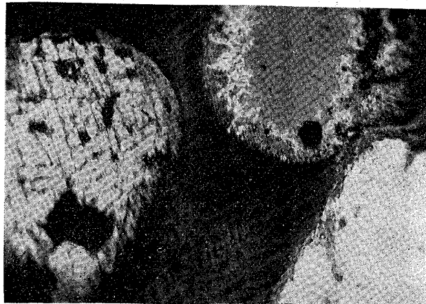
No. 9 × 250 Iron sand from Aomori, reduced at 911°C for 2 hrs. with CO gas. Red. %..... 89.52
