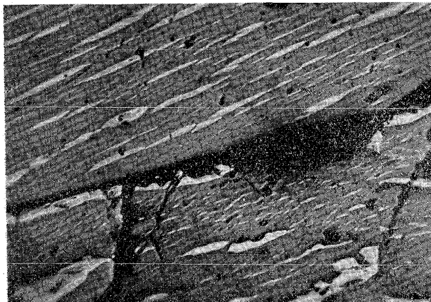
No. 22 × 100 Ilmenite from Ekersund, Norway not etched.
