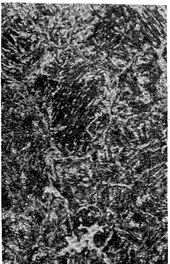
No. 12 Mo 1%, C 1.4% 1,000°C より爐中冷却 ×400
