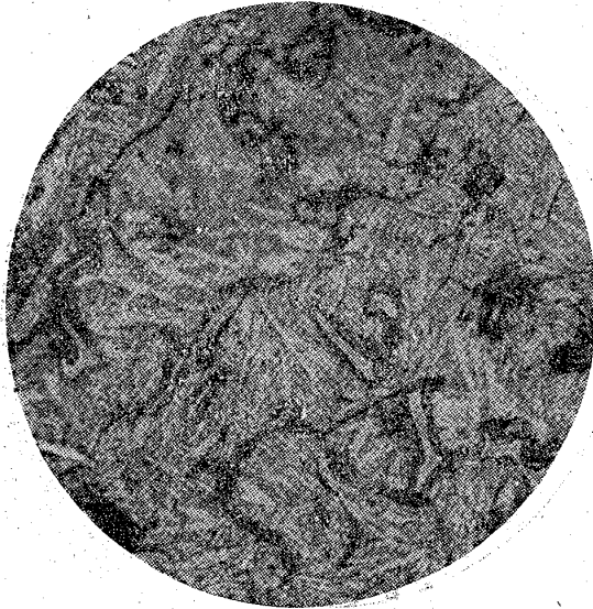
× 100 Etching by picric acid No.14
