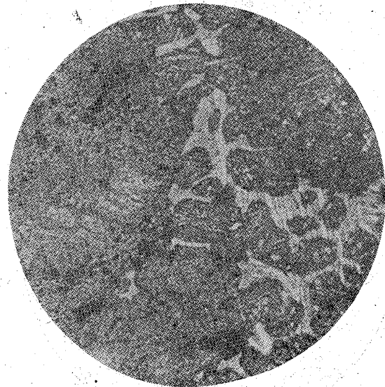
× 100 Etching by picric acid No.17
